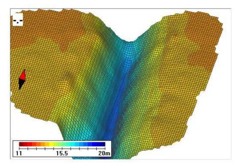
To get a value for Tilt you can repeat the process (with the value for Latency found above), but with a measurement from considerably deeper water (>40m). If you are not going to map details in deep water (such as ship wrecks) you do not need to worry about Tilt - just set it to zero.
